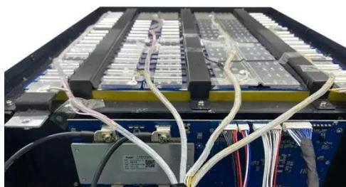
17 hours ago BESS (Battery Energy Storage System) is an advanced energy storage solution that utilizes rechargeable batteries to store and release electricity as needed. It plays a crucial ...
