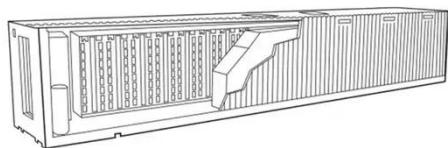
The 200KW Solarfold Mobile Solar Container from HighJoule features a foldable deployment system using 610W modules. It's a high-yield, portable solution for urgent deployment and ...
