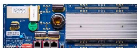
RS485 Communication between battery and inverter Band rate 9600bps RS485 Interface Communication between profile packs or BMS and PC Band rate 9600bps
