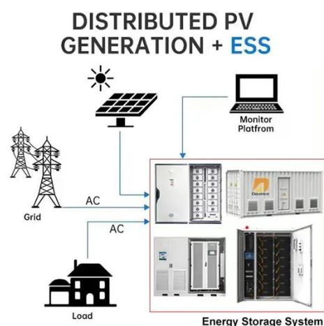
Standardized Battery Modules, the Battery Management System (BMS), the Power Conversion System (PCS) and Energy Management ...
