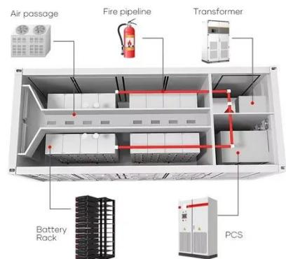
**500kW/1000kWh Lithium Battery
