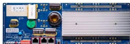
RS485 Communication between battery and inverters Baud rate: 9600bps RS485 Interface Communication between parallel pumps or EMS and PC Baud rate: 9600bps
