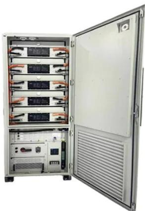
battery as energy storage, automatically charges and discharges via a bidirectional converter to meet ...
